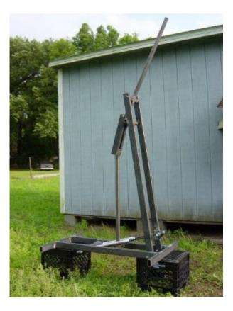
The rod clevis' are attached to home made brackets. Generally, the clevis "sandwiches" the bracket and a pin fitted with external snap rings secures the joint.
