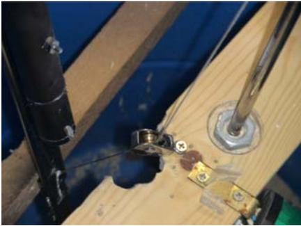
Make sure the string does not abrade rubbing on surfaces.
