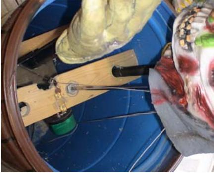
A pulley is attached to feed the string from the base of the head to the bottom of the drawer slider
