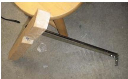
18 inch drawer slider has L bracket on the end
