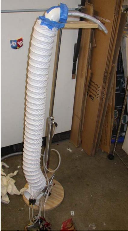
In the extended state, the vinyl dryer ducting takes the glycol fog into the head/mask without much condensation loss
