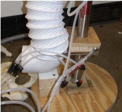
The 2.5 inch PVC elbow was used to channel the fog from the fog machine into the flexible vinyl dryer ducting.
