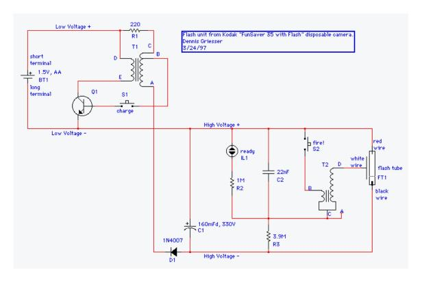
This particular circuit contains two gas discharge tubes. Understanding how they function is the key to operation of a strobe light, and how they might be useful to the haunter.
