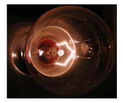
This photo of an incandescent lamp with a clear envelope shows the filament glowing white hot.
