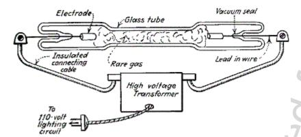
This drawing of a simple neon tube is from *Neon Signs*, by Miller and Fink, a 1935 text on neon lamp manufacture.
