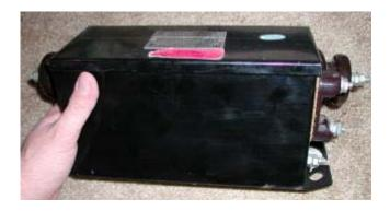
This is a traditional neon sign transformer. It puts out 12,000 Volts at 30 mA, and weight 19 pounds.
