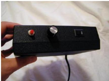
The front of the controller has: test switch, sensitivity control, and power switch. The power switch also contains a pilot light.
