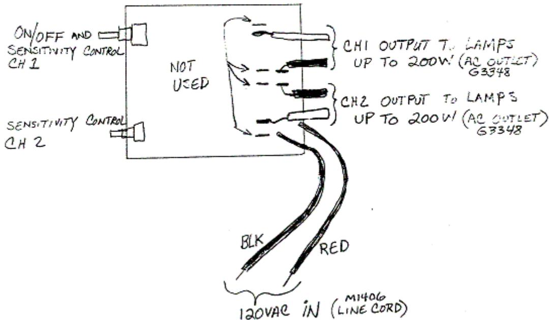
① IT'S A GOOD IDEA TO ADD A 5AMP FUSE IN SERIES WITH THE POWER INPUT RED LEAD
