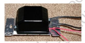
Be sure to clearly mark the wires that you added, because they will have to be connected to the photocell eventually.
