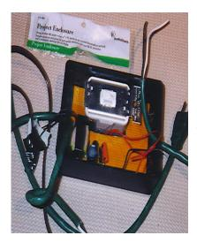
Here's the LLB under construction. Note that I fit the entire dimmer box inside the project box. It's neatly laid on top of the perf board mounted electronics shown in schematics. I had to shear off the dimmer light switch to get it to fit in the project box, but no matter...no one is going to need it. I just moved it to the full "on" position. With the photocell to regulate the output through the triac gate, this works great!
