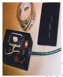
Here's the LLB completed with the top off the project box. Note the JB Weld epoxy around the extension cord hole in the side of the box. As an additional measure, I always put a knot in the cord just inside the box as strain relief in case it accidentally gets yanked. Finally, I use clear package storage tape to seal the box after the top is screwed on. Four pieces of tape to cover the small gap around the edge.
