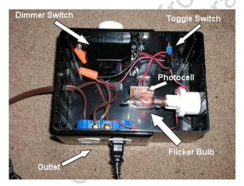
6) Wire all the components according to the schematic below:
