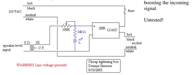
Components in blue are optional, but highly recommended. The transformer output is AC and the SSR input is DC. Half the time, the LED will be reverse-biased. The optional LED, in addition to serving as a pilot light, gets rid of the reverse bias on the LED inside the SSR.
