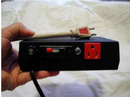
This is the rear of the control box, showing: fuse, speaker-level audio input, indicator lamp, and socket for the flash head.
