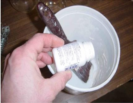
Remove the glass globe and apply the etching compound as per the instructions on the label.
