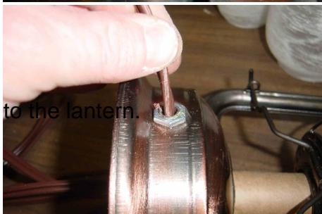
Now we'll need to secure the other threaded rod and nut to the lantern. Doing the same thing we did with the washer assembly by putting the epoxy on the back side if the nut. Pushing firmly, press the nut on
