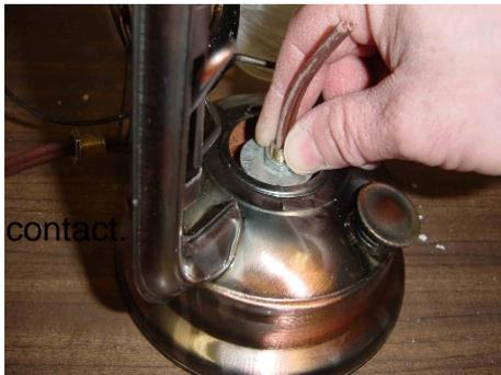
Push the cord and washer assembly back into the wick opening.
