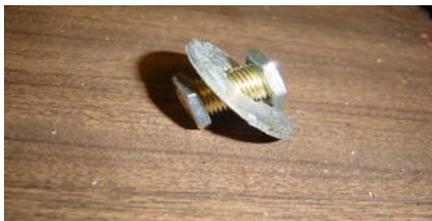
This is similar to what we did a couple of steps ago. This time we'll place a washer between the 2 nuts and tighten leaving enough thread on end to attach the socket.
