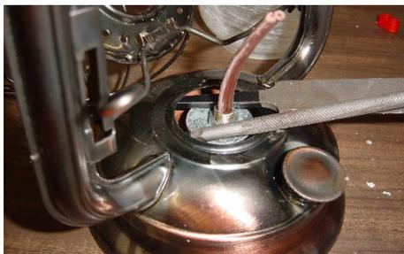
Using a screw driver, file or what ever will fit, to hold the washer in place until is dries.
