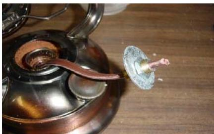
Time to place this piece on to the cord. Leave enough room so that you can flip this upside down to apply the epoxy.
