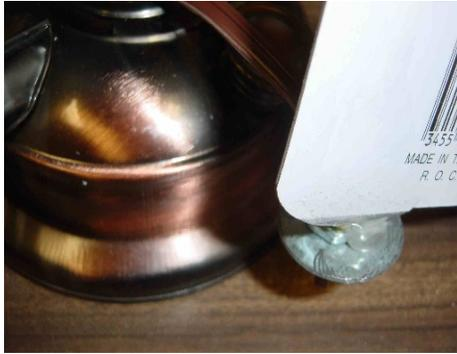
Mix the epoxy as directed on the label then apply to the back side of the washer.
