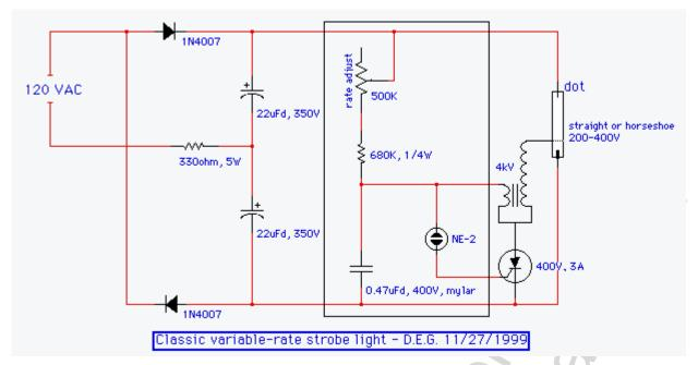
Here's a simple strobe, with the relaxation oscillator near the center, enclosed in a rectangle.
