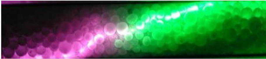
The power supply turns on and off at a rate that you can set. Each time the power comes back on, the electricity finds a new best path to ground.
