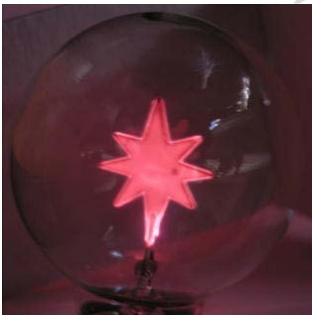
This display results from flat plate electrodes in the shape of a star.
