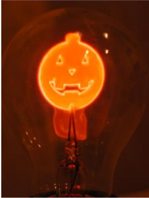
This display results from [flat plate electrodes](#) in the shape of a pumpkin, with cutouts for the eyes, nose, and mouth.
