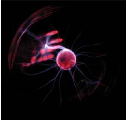
Placing your hand on the sphere attracts the electricity. Your body provides a mild path to ground.
