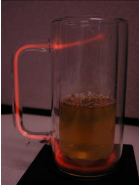
This clever toy from [Can You Imagine](#) forms the glass envelope into the shape of a mug. The mug is free to move around, and only lights up when it sits on a small battery-operated "coaster".
