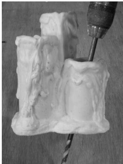
A pocket is drilled out on the bottom of the candle set base using the 1 3/8" bit. Make it deep enough for all the wires to be stuffed into.
