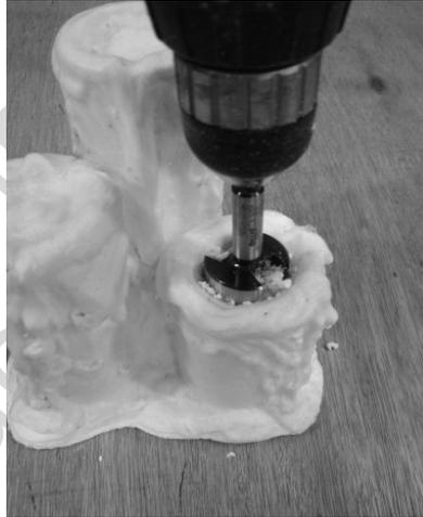
Using a 1 3/8" bit as shown, drill out each candle that will have a socket installed in it. Drill deep enough so that the top edge of the ceramic socket is just below the foam.
