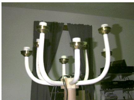
After I got all my arms made I put them together. To do this I made a kind of tinker toy for the center out of a block of wood. I cut the block into a hexagon and drilled holes to accept the arms. Using the sockets and socket holders from the light kits I wired each up and connected into a single line.
