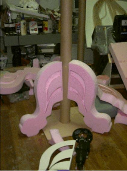
For the stand of the candelabra I started with a cardboard tube. I mounted these to a 12" square of thin plywood. For the legs I made a pattern out of cardboard and then traced it onto a sheet of insulation foam. I cut these out, and using a dremel tool I carved the decorative designs in the sides. I sanded the legs with 120 sandpaper to get a nice smooth and rounded edges. Using liquid nails I glued these to the cardboard tube.
