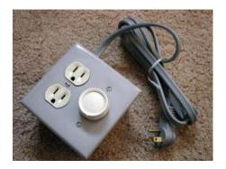
The complete dimmer box gets power from a standard three-prong plug. It has two sockets to feed your lights, and a knob to set their intensity.
