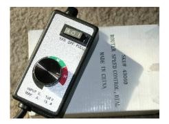
This unit, from <u>Harbor Freight Tools</u> (#43060), is sold as a motor speed control for a router. It will also function as a lamp dimmer, handling a load up to 15 Amps.
