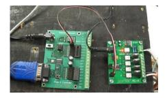
I haven't put the FC-4 into a project yet but have played with it using a Prop-2 controller. As you can see in the photo to the right, the connection between the Prop-2 and the FC-4 is just one jumper cable.
