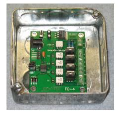
For the lighting controller I originally built, I put all the "high voltage" components into a closed box for safety. Since the FC-4 involves high voltages, I recommend that it be installed in your project where it can't accidentally be touched. As you can see from the picture at left, it fits nicely into a two gang electrical box. (If you're going to mount it in a metal box, be sure to use insulating standoffs so that the circuit board doesn't touch the box.)
