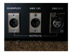
Here is the output of the Sunn PLC 3200 control console. It sends exactly the same information in three different formats (it also speaks MIDI). We are interested in the DMX output to the right.
