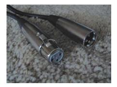
Here is the connecting cable. It is male on one end and female on the other.
