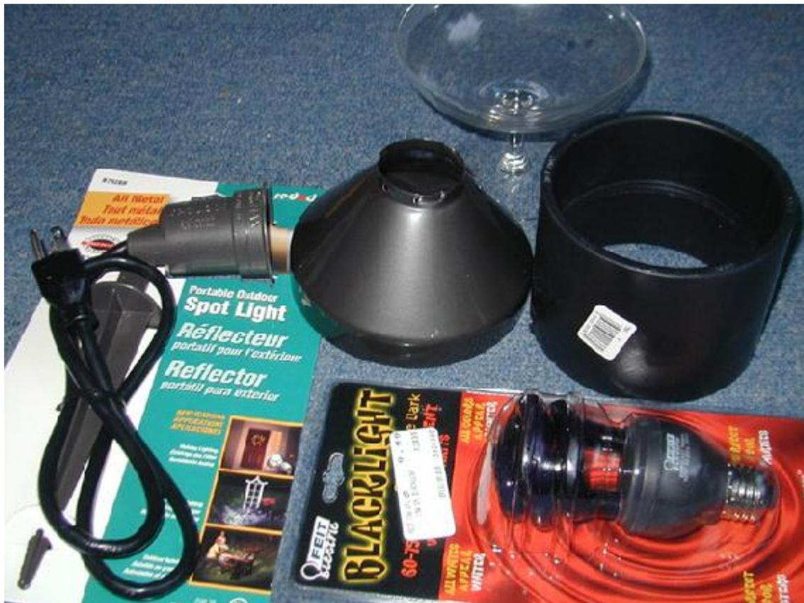
Components: Outdoor garden fixture, Feit Fluorescent Black light (Fry's), cone from motion sensor kit, 4" plumbing union connector, margarita glass
