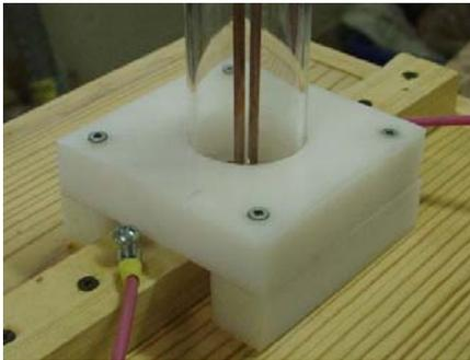
The white plastic stuff is Tivar 1000. We use it at work and I was going to try to put the copper rods in that but at times this stuff would catch fire and start to melt when the arc started so I dropped that idea and went with the 2x4. Although it worked great to secure the acrylic tube in place. I'm sure you could use any kind of lumber if you decided to build one like this
