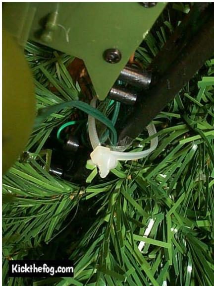
Remove the mouth plate from the 2 mouth plate mounts. As you can see I removed all the branches and stuff from the mouth plate but this was not necessary as we are not going to use the mouth plate for anything anyway.
