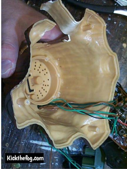
You are left now with an empty tree trunk with just wires running through it. We need to remove the wires from the trunk so we can discard the trunk.
