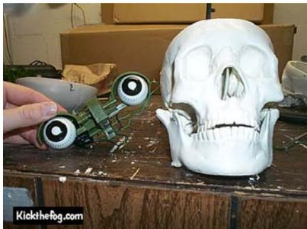
Test him! If the tension is correct, the servo will pull the jaw open. If it's too tight the jaw will not open. If the tension is not high enough, the jaw will open and stay open. Adjust till jaw opens and closes correctly. To do this you can plug in the tree and let him belt out his Christmas Songs. It's pretty damn funny to see a skull sing Christmas songs so I suggest
