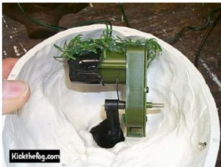
This is the desired end result. Pic1 is of the mounted servo with the arm on the servo sticking out the hole. Pic 2 (ignore the springs, pictures taken out of order) shows the bottom
