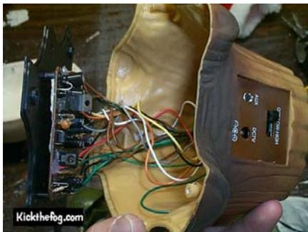
Remove the screws that hold the bottom panel of the tree. Carefully remove the panel with all the crap attached to it.
