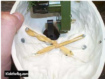
This is a view of the completed jaw tension setup. This is where you have to experiment a bit. I played around with the rubber bands by tying and untying knots in them to increase and decrease the tension. Adjust them so that the jaw stays closed BUT so that only light pressure is required to open the jaw. THIS IS CRITICAL as the servo doesn't have a lot of gusto.
