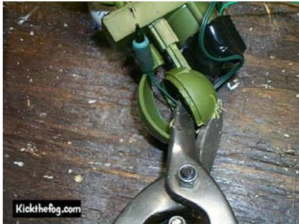
I used a pair of tin snips (pic 1) to cut the socket so I could slide the wire free without breaking or disconnecting the wire.
