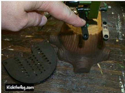
Here is an earlier picture I took. Ignore the trunk which has already been thrown out at this point. Notice the mouth. I removed the screws that hold the plastic mouth to the arms of the servo. Throw the mouth away.
