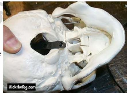
view of the mounted servo arm. Picture 3 shows my second servo mounting hole drilled. In goes the screw and off to the next step!
