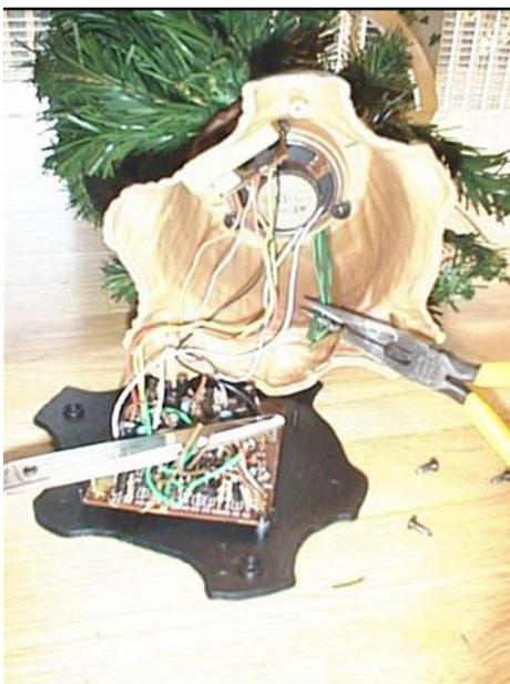
Remove the screws from the bottom of the base and cut the wires close to the electronics in the base.
