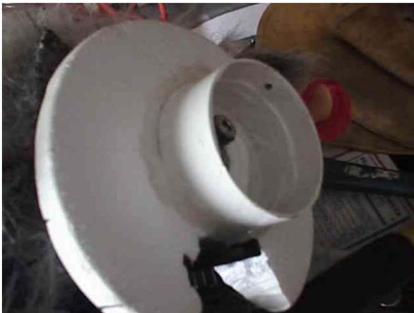
**I've taken a 2" PVC joint (the inside diameter is just under 2 1/2") and used a saw to cut it in half. The connector was about 4-5" tall and I didn't want that much neck.**
