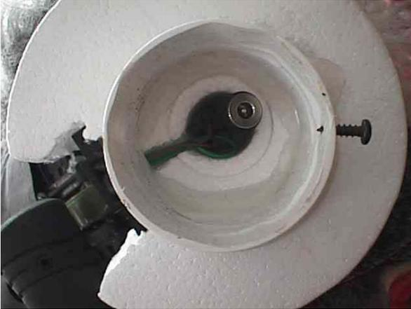
Here you see the view from the bottom of the wig head. You see the connector that will plug into the Santa neck connector and a small screw I added to tighten after the PVC is slid over the Santa neck stump.
