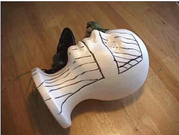
I've marked the section of the foam head I'm going to remove with a hot wire foam cutter.
