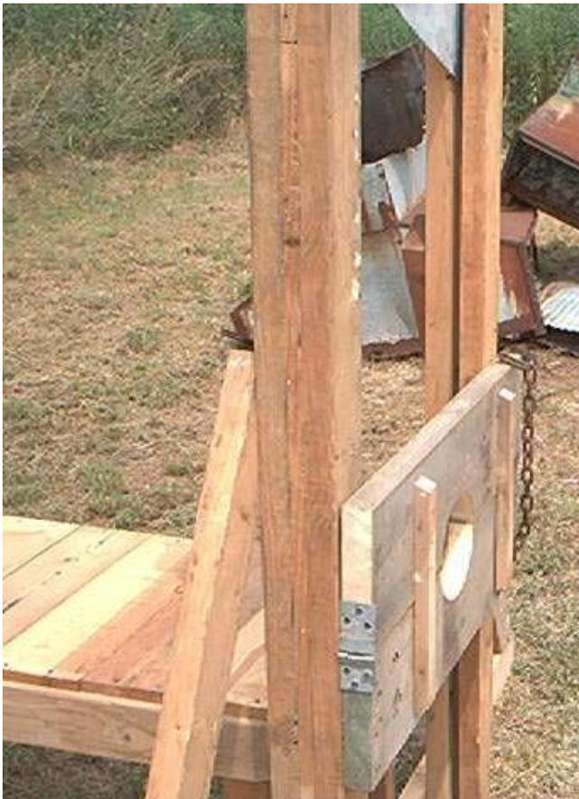
Here's a side view showing the hinge. You can also see the track for the blade. The blade track is 3/4" wide. The blade is made out of 1/4" AC plywood that has been painted with chrome color paint. It moves fairly easy in the track. I cut the whole in the stock with a saber saw.
