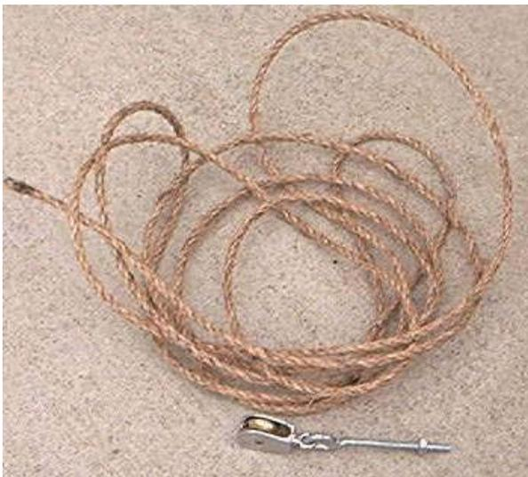
Here is the pulley and the rope. The pulley is attached to a 4" eyebolt that will be fastened to the top 2X4 of the guillotine
