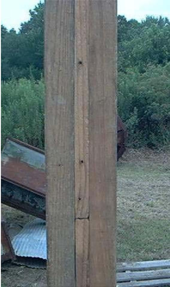
The guillotine blade tracks are made from 2 2X4s nailed face to face with a strip of 1X2 lumber at on edge between them. This gives you the 3/4" gap for the blade to run up and down in.
