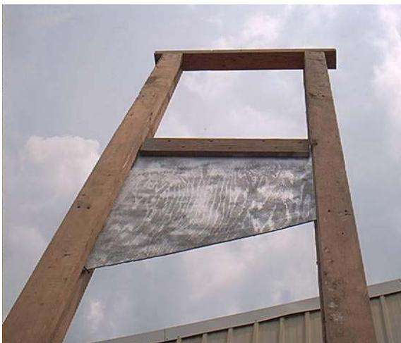
The blade has 2 1X4s screwed together on either side of the blade. They are about 1/2" from shorter than the width of the blade track to keep it from binding.
