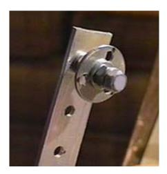
The image at left shows the holes drilled into the finder washer for attachment of the marionette control lines. Be sure you adjust the nuts so that the fender washer can spin freely but not wobble. Be sure to oil the pivot with a light oil, such as 3-In-1. Admittedly, this is hardly an industrial part, but it moves slowly and will work for many seasons before needing replacement. It is very inexpensive, and you can always build a spare to keep on hand.
