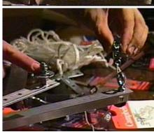
The arm pulleys attach to eyebolts mounted at the ends of the arms as shown, using nylon twine or tiewraps (which make it much easier). This allows the pulleys to twist as the crank changes position. The control lines for the marionette's arms lead through the pulleys to the crank pivot. The pulley wheels should be reasonably close to the plane of the pivot when the lines are under tension.
