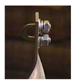
For attachment to the motor shaft, you will need to drill two holes in the crank arm, spaced to accept both legs of your small U-bolt. It is important to make sure that when the bolt is attached to the motor shaft, the aluminum does not drag against the platform members. The clamp attaches as shown at right.
