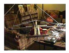
The image at left shows the motor platform with the control lines installed. The thick lines should be blackened with a permanent felt tip marker to keep them 'invisible.' If you want to keep the lines to your marionette thin, cut the lines such that they hang just below the pulley when the crank pivot is farthest the pulley for each line.
