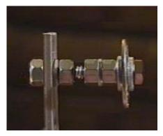
The pivot at the outer end of the crank, to which the control lines attach, consists of nothing more than a bolt attached to the bar through a hole, with a wide fender washer that is set so as to spin freely, using the bolt as an axel. The fender washer has three holes drilled with equal spacing around its perimeter, forming the attachment points for the lines leading to the marionette's head and arms. The part sequence is illustrated in the photo at left; left to right:
