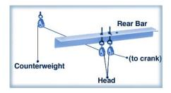
The mounting eye for the pulley supporting the marionette's head attaches to the center of the rear cross member. We use an eyebolt with a 4-inch long shaft, and locate the eye below the frame, where the head pulley can be attached. The top of this long bolt - extending above the frame - is fitted with a fender
