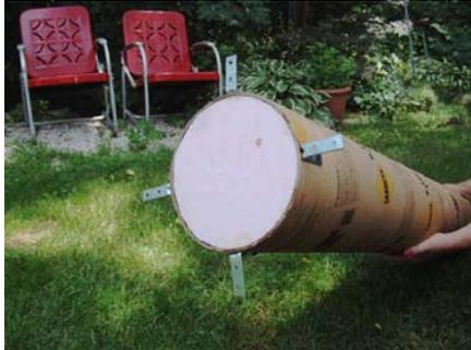
Find and mark the exact center of the top of your wooden box. Stand the tube up onto the box and drive screws through the brackets. Glue around the seams and brackets for extra support. Apply some more glue to the bottom of the base foam, fit it over the tube and brackets; Once seated, use screws to fix the base.
