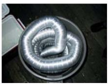
Since the aluminum dryer hose came in 6 foot pieces we had to attach them together using 3M Water Resistant Duct Tape. Then we put on end of the tubing out of the lower (exit) hole and coiled it around the inside of the can. Once we got to the top we fed the tube back out the higher (enter) hole.
