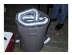
Here's a side angle of the chiller. The tube coming out of the right is the one where the fog goes in. See, all done. Quite simple yet very effective. The fog has to go through 18 feet of tubing. That's a lot of cold going on!
