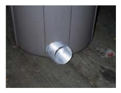
The great thing about the garbage can is the material is much thinner, I'd just score it a bunch of times with an x-acto blade instead of buying the 4 inch bit. The hole where the fog comes out is right at the bottom and the hole where the fogger nozzle is placed it about 2 inches higher on the other side.
