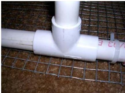
Using the 90 deg and T fittings, join all the pieces together and check for fit in the cooler. Once you are happy with the fit, bond everything using PVC glue.
