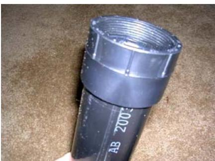
Two pipes are needed to get the fog from your fogger into the system, and direct the chilled fog out of the system. The inlet pipe consists of three pieces: A female 2" threaded/slip Black ABS fitting, a 2 1/2" piece of Black 2" ABS pipe, and a 2" Black ABS Y
