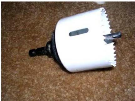
You will need a 2 3/8" hole saw to drill the holes in the cooler. The hole saw cuts through the cooler like butter so go slow, and make sure you line the drill bit up so its level.
