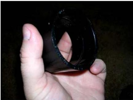
You will need a 2 short lengths of Black ABS pipe cut - figure 2 1/2" each. Take your PVC primer and glue and glue a male 2" threaded/slip fitting on the end of each 2 1/2" piece of pipe.
