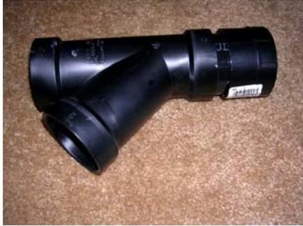
pipe. Glue the Y pipe with your PVC glue to one side of the 2 1/2" piece of pipe, and glue the fitting to the other side. This forms the inlet pipe.
