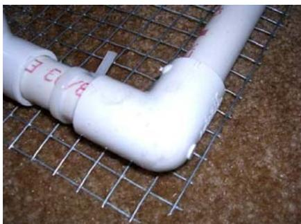
Next break out the hardware cloth (chicken wire like mesh) and cut a piece the same size as the PVC tray. Zip tie the mesh onto the tray. Insert the completed ice tray into the cooler and check for fit.
