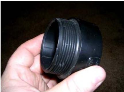
Now take the coupler fittings and glue them onto the portions of pipe that extends into the cooler. Make sure you push the pieces together to get a nice tight fit. Use your caulk around each pvc pipe to make a nice seal with the plastic of the cooler and your fittings.
