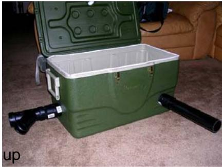
The Fog on the Rocks chiller is a great design by Deathlord. Its cheap to build and works really well. Throw in a couple bags of cheap cube ice and you can chill fog for hours. The particular chiller design works best with fog machines under 700 watts. If you have a larger fog machine, you should check back in a few weeks for a larger garbage can based chiller I am building right now. I plan on putting a full how to on the web for it soon. Anyway.. lets get building.
