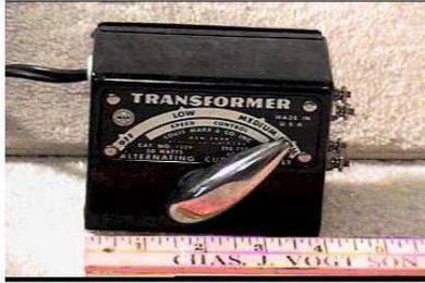
I purchased my vintage model train transformer on eBay for \$7. You may have a better alternative for a power source, but I recommend you use one with a variable voltage control. Also, newer models have circuit breakers built into them that disqualify them for use in this application, so older power supplies seem to work best.
