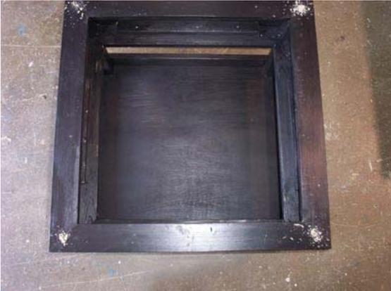
Using either scrap or new lumber, construct a box to house the fan and paint it black. Since the dimensions of the box will differ depending on the size of the fan, exact measurements are not given. Take notice of the small "lip" inside the box which supports the fan.
