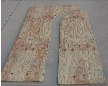
First, I measured out the first door and cut it out using a jigsaw, after I cut out the FIRST door, I placed that half of the entrance archway onto the other piece of plywood and traced the outline. Why did I do it this way ? So that the doors would be identical to each other!
