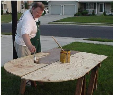
After the doors were cut out, I stained and polyurethaned the doors ( 3 coats ) to protect them from the elements and to give it a nice 'wooden' appearance.
