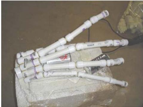
I put an all-thread rod through each finger. The rod can be bent to any desired configuration or look.
