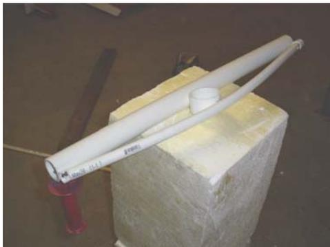
The arm is composed of a 1 1/4" and a 1/2" PVC pipe. The 1/2" pipe is longer than the larger...if you bend the pipe around an object and bolt it on both ends it will remain in a bowed configuration and look similar to real arm bones.
