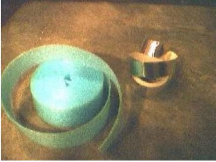
For the conductor, I used aluminum heating duct tape, also from Menards for ~ \$5.00.
