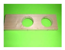
(1) Saw a piece of 1 X 3" wood making it 7" long. Measure 2" from one end and mark that spot in the center of the board. Using a hole saw attachment on your drill, cut a 1 + 3/4" hole. Repeat these same steps on the other end of the board. This will make the eyes exactly 3" apart (center to center).
