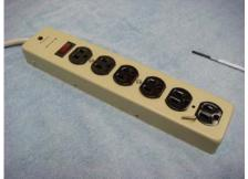
Make room for the sensor by taking out the last receptacle
