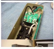
Find the wires that go through the switch and cut them open to splice in the new switch (which is the motion detector) all the wiring set-ups are in the directions that came with the motion sensor.
