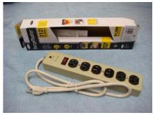
I like to use this type of power strip because it's metal and easy to take apart and put back together. Also has surge protection, an on/off switch, and power on light
