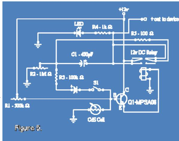
Adjust the time period with R2 (Radio Shack #271-211 \$1.50) which shortens the time period by charging C1 faster, or leave out R2 and simply change the size of C1. A 470µF capacitor (Radio Shack #272-1018 \$1) can give up to 60 seconds, but that will vary depending on the transistor. The time period is sensitive to the adjustment of R1, so adjust R1 before adjusting the time period.
