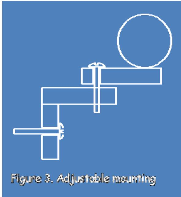
Figure 3. Adjustable mounting
