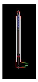
If you're looking for a fairly inexpensive way to build long throw pistons (12 inches or more), then the PVC pneumatic piston is the way to go. They're powerful enough to lift about 10-15 lbs at 40 psi and only take about 1/2 hour to make if you have the proper parts & tools on hand.
