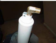
Once I had the end of the piston threaded I test fitted the elbow that I picked up while on my search for parts.
