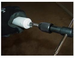
Next step was to drill out the existing hole and tap it for a 1/8 inch pipe thread. I kind of guessed at the pipe size while I was at the store and it turns out that 1/8 inch pipe thread is perfect for the hole.
