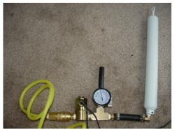
The assembly you see in the image to the right is what I ended up with. I connected the 55 PSI hose connector to a small electric valve that I picked up a few years back from a pneumatic supply shop. I attached that to a T fitting and ran it through to the piston.
