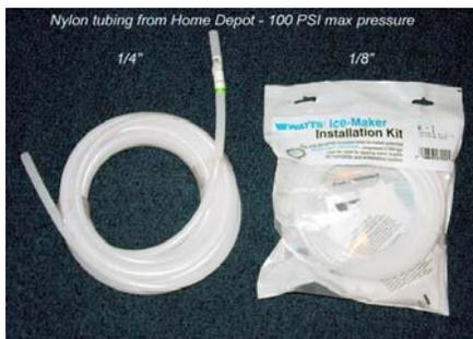
By using nylon pneumatic tubing and quick-connectors to hook up your devices, you will have a set of components that plug together as quickly as Tinker-Toys. This tubing can be cut with a razor knife to any length desired - just be sure to make your cut clean and straight. *Remember, the measurement given for this tubing is the **inside** dimension, not the jacket; and that is also true of the fittings and adaptors discussed below.* This is often confusing to first time
