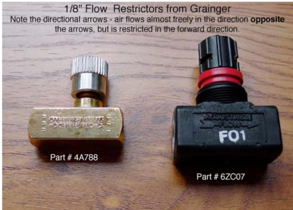
What are they used for? Making an animatronic move at the proper speed, for one thing. Pop-ups often reset as violently as they pop unless a flow restrictor is used on the exhaust cycle. Sometimes one is needed on the activation as well. Remember, violent action is what kills props ahead of their time, so here we have a means to avoid it. Grainger has them, as shown in the image above.
