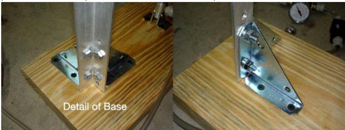
Here's how the completed base should look with the upright and corner brackets
