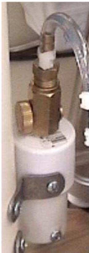
NEW! The new "compact" muffler shown here uses 1" PVC pipe just 2 1/2" long with one end capped and threaded for the valve you see installed.
