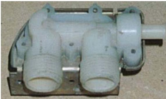
Of course you will need a water valve from a washing machine and not just any valve will hold the air back and reseal itself under the rather high pressure I would need for an air cannon. I wound up testing many, many different valves to see which work and which don't.
