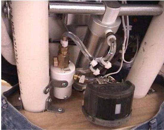
Here is yet another way to use your compact muffler. These photos, which was first used in the 2003 project, the [Lynching](#), shows a second fitting on the top side of the muffler that can be used to silence the exhaust from the secondary air inlet on a 2 way air ram. You must route these two lines into the muffler separately, as if you link them together, you will in essence be attempting to force air into both the PUSH inlet and the PULL inlet of the same air ram.
