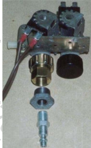
Slip on to either lead on the solenoid that triggers your water valve and then cover each with heat-shrink tubing or electrical tape. It does not matter which power cord lead you send to which connector. Either way will work as long as you attach your air nipple to the corresponding cylinder .
