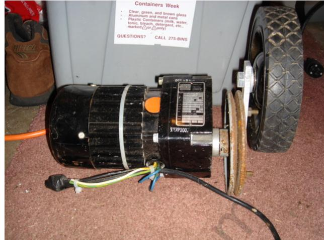
The first step is finding a motor that handle this type of load. The motor that I used was Bodine 1/15 hp with 10 RPM motor from C & H Sales Company. You can find them in my Links page. This motor has a 5/8 shaft and also has a hole drilled through the shaft. The arm is a piece of aluminum that is 1/4 inch thick and 7 1/2 inches long. The arm attaches to the motor using a 5 inch diameter V-belt wheel. The other end of the arm which opens the lid has a 6 inch lawn mower wheel attached to it.
