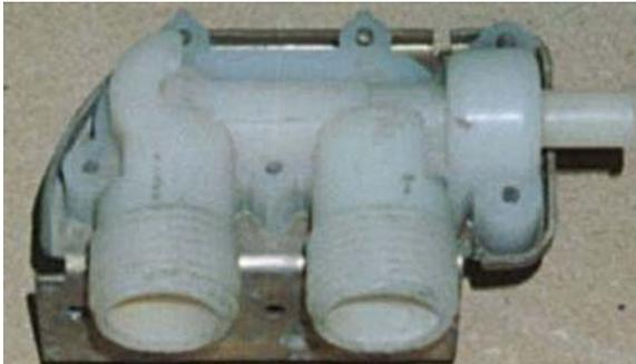
Of course you will need a water valve from a washing machine and not just any valve will hold the air back and reseal itself under the rather high pressure I would need for an air cannon. I wound up testing many, many different valves to see which work and which don't.
