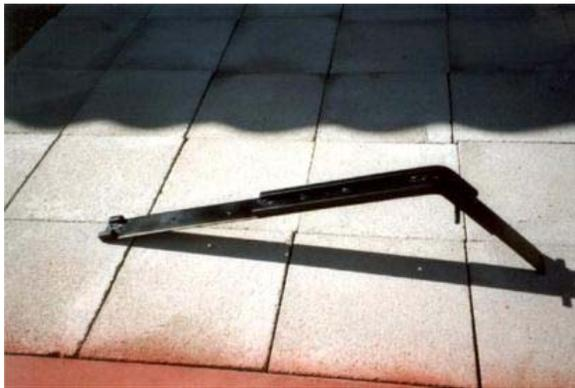
I went to a metal shop to have my 1/8" X 2" X 28" lever bent and an axle pin welded on to it. Instead of using a heavy 1/4" thick stock I chose to reinforce the more stressed section of the lever with some 1/2" square metal tube as you can see here to keep the weight down. The small sections of the square tube seen at the left end of the lever were put there to achieve another idea I was working on that I abandoned, so you need not address this.
