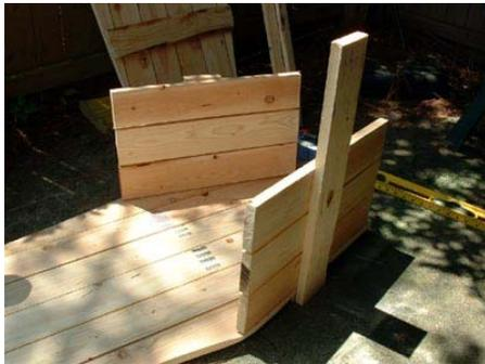
Build the 4 sides using 3 boards each this time. The short sides are 18.5" long and the long sides are 30.5" long. Add a perpendicular 10" down on the short side and 12" up on the long side. Make sure that you allow this board to overlap 1.5" on each side so that when you put the top and bottom together, the perpendicular boards will be flush. You will need to cut 1" X 2" strips to install on the opposite inside of each side to hold the boards together.
