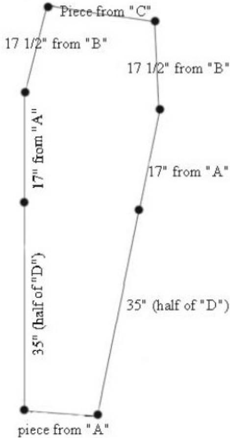
This sketch shows how to cut the A, B, C, and D pieces so they will fit around the coffin bottom.
