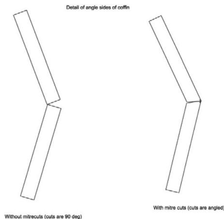
Without angled cuts where the sidewall segments meet each other, there will be a gap on the outside. The exact angle of the cut doesn't matter, as long as the two segments can touch on the outside. A gap on the inside is easier and neater to fill (with caulk, putty or epoxy) than the outside is.
