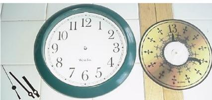
**EVEN MORE CAREFULLY** remove the second hand, then the minute hand, then the hour hand.
