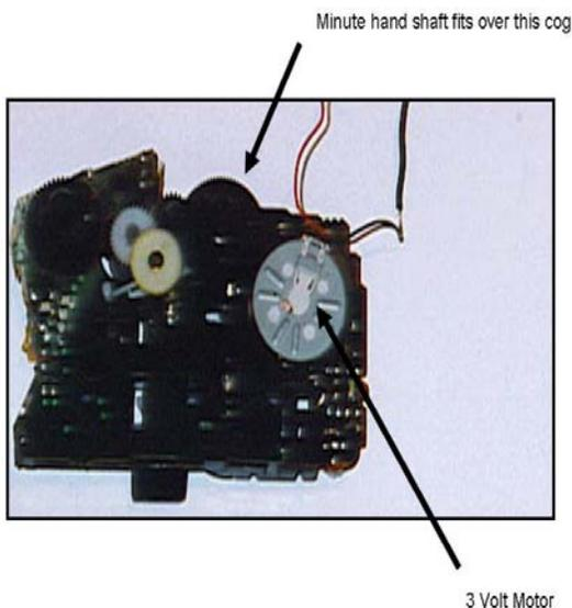
What you'll see is a little 3 volt motor that drives two rubber pulleys with a bunch of gears to reduce the speed.
