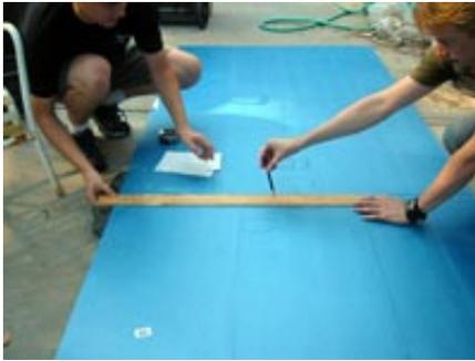
Here you can see us measuring and drawing our designs with a grease pencil. We cut the foam into thirds length wise, then 2 of the 3rds into more thirds, and the last 3rd in half. This gives us 8 pieces. Actually, we cut one of the pieces a little taller with it's top being the sides of the pieces cut in half. The foam we got came with some platic coating which we peeled off. Sometimes it would come off nicely and other times it would be a pain.
