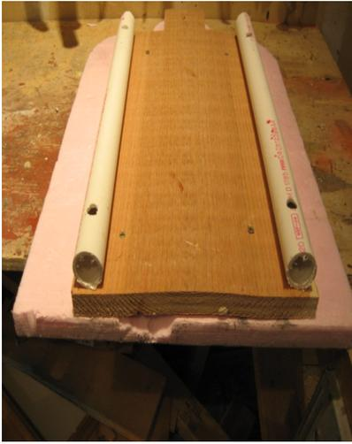
I then used a cedar board glued to the back of the styrofoam board to keep it stable in the wind. A couple of lengths of 1/2" PVC pipes screwed to the back. This allows a place to slide in your rebar. This rebar is pounded into the ground...to hold the thing up.
