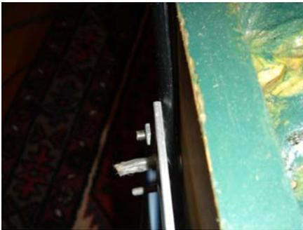
Take the other screw and put it into the bottom hole of the stake in a way so when you attach the stake to the wood the head faces the wood and then tighten a nut on the screw. The bolt that you attached earlier to the wood you will want to add a couple of washers to. This will help give a spacer between the wood and the grave. Next attach the stake to the bolt attached to the wood.
