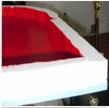
We attach 2" thick Styrofoam (using a low heat hot glue gun) along the edge of the back piece. Placement along the edge does not have to be exact, since we will trim it later, but you should make it at least cover the edge of the back piece.
