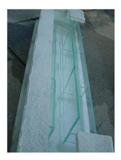
However, when it was first tried outside, wind moved the Styrofoam back and forth causing it to dig into the fins, so pieces were added between the fins. Holes were notched out of the bottom spacers to allow the water to flow back to the pump.
