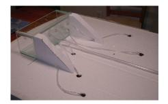
At first the tubes were placed inside the holes, but the water shot out of the holes and could not be contained.
