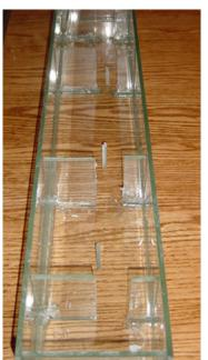
1/4" Plexiglas was used for the tanks which provided a stronger tank. The lower tank is the only thing that supports the stone.
