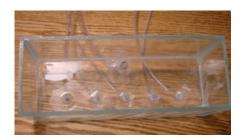
The upper tank has one  $\frac{1}{2}$ " feed tube and five  $\frac{1}{2}$ " tubes which feed the bullet holes.
